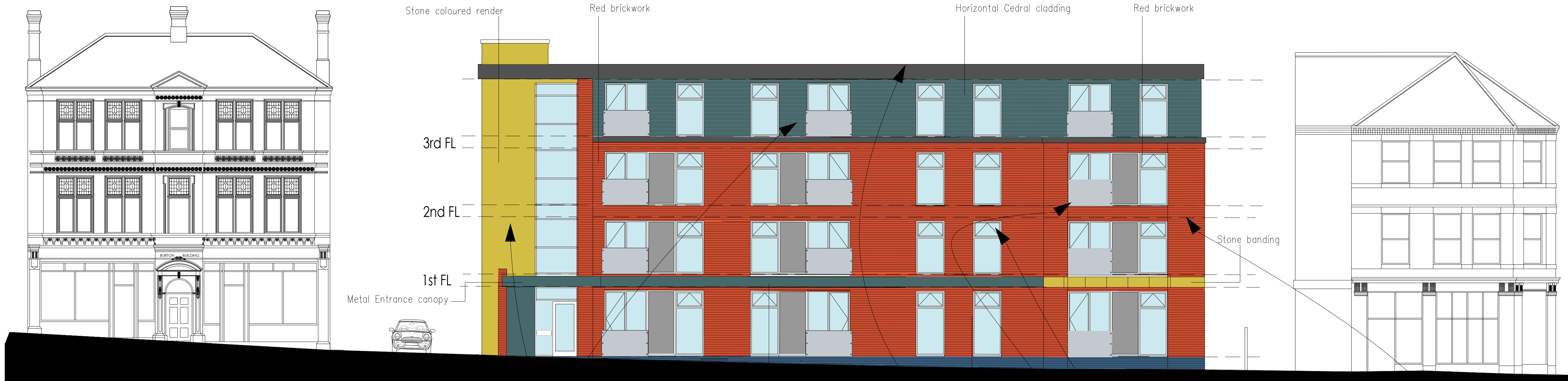
PROPOSED FRONT ELEVATION TO BRIDGE STREET. 1:100
