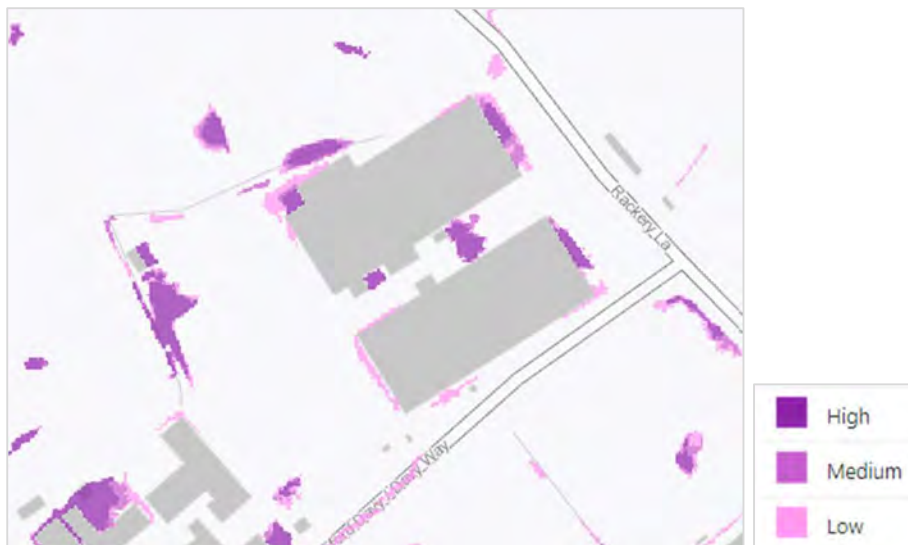
Figure 7 – Flood Risk from surface water and small watercourses (extracted from The Development Advice Map – Natural Resources Wales website).
