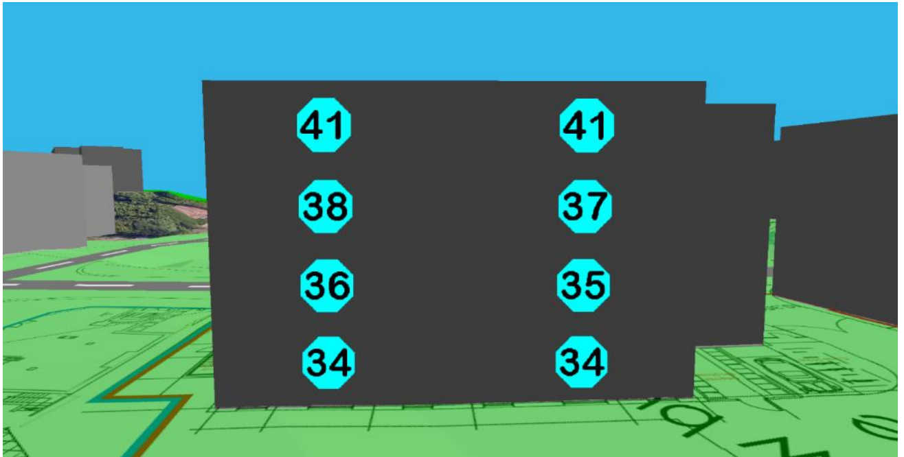
Façade B – Night-time Road Traffic Noise, L_{Aeq, 8hr} dB (Buildings removed for visual purposes)
