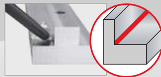
Inner Straight Corners For Sets: G3
