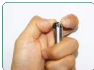
Slide the drill insert into the slot of the holder and press down the insert to touch the bottom of the slot.
