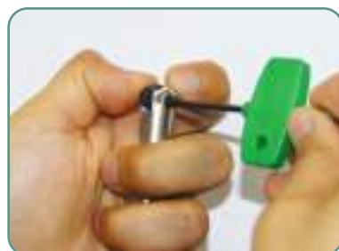
After confirming the insert is pressed down to the bottom of the slot, tighten the screw using anti-seize compound.
