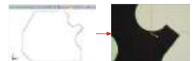
Input CAD drawing and set reference, move the stage to make the target box in the center of crosshair, then the software will do automatic measurement
