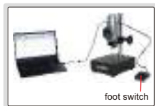
data transmitted to Excel without software
