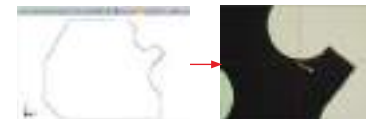
Input CAD drawing and set reference, move the stage to make the target box in the center of crosshair, then the software will do automatic measurement
