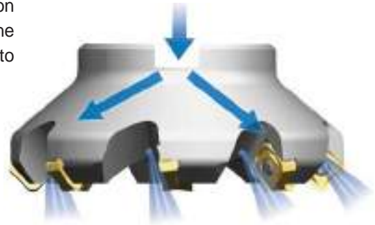
Through coolant system for decreasing cutting heat and good chip evacuation
