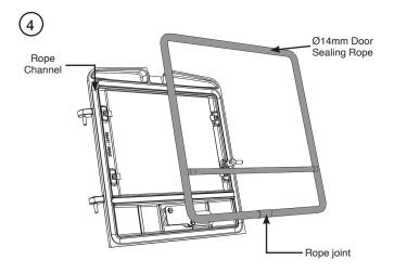
Remove the old rope and scrape old glue from the locating groove.
