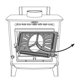
The Door Tool can be used to remove the Ash Pan.
