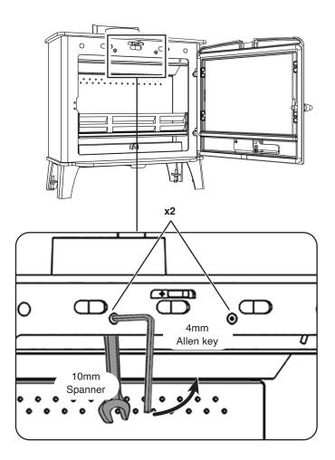
Loosen the hex bolt until the slider moves with no resistance. Once happy with the sliding action tighten the 2 locknuts.
