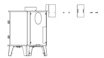
Align the Heat Shield on the slots to cover the gap between the Twin Wall and the Top Plate. The overlap must be at least 10mm.
