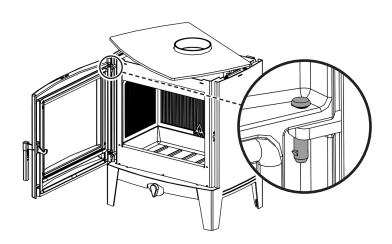
Rotate the hinge pin with pliers if the retractable barb is not showing.
