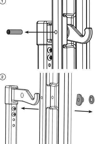
Replace the handle. Ensure the washers are replaced in the correct order.
