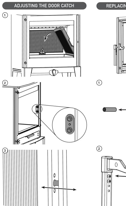
Fully tighten the nuts to secure the Catch.
