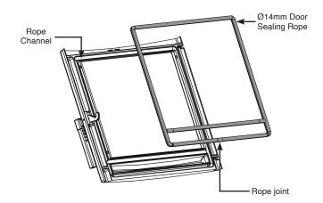
Remove the old rope and scrape old glue from the locating groove.
