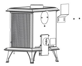
Align the Heat Shield on the slots to cover the gap between the Twin Wall and the Top Plate. The overlap must be at least 10mm.
