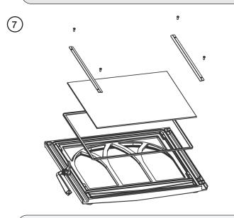
Take note of the roping around the edge of the door glass around the edge. This will also need replacing.
