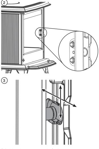
Fully tighten the nuts to secure the Catch.
