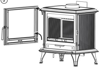
Lay the door face down on a soft flat surface, to protect the paintwork and glass.
