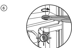
To release the pin, retract the barb using flat pliers and pull the pin upwards.  $\,$
