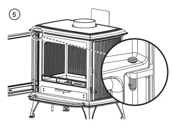
Rotate the hinge pin with pliers if the retractable barb is not showing.
