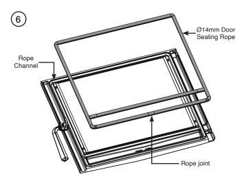
Remove the old rope and scrape old glue from the locating groove.
