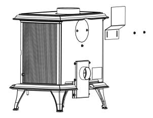
Align the Heat Shield on the slots to cover the gap between the Twin Wall and the Top Plate. The overlap must be at least 10mm.
