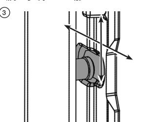
Fully tighten the nuts to secure the Catch.
