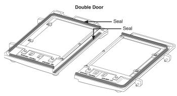
Clean the locating groove with a clean, dry cloth to remove all old dust and debris.
