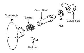
Check the door catch operation and tightness of the lock nut. Adjust if required.
