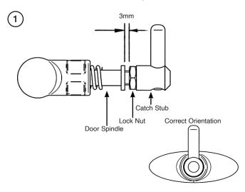
Screw the catch stub up to the lock nut. Ensure the correct orientation of the pin and knob.
