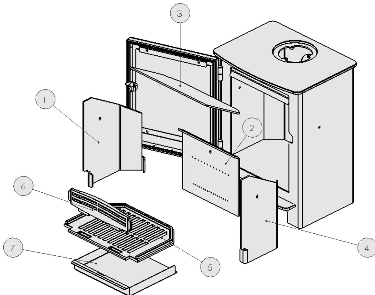
To refit the internals follow the numbered sequence from 1 – 7. The rear firebrick should be fitted with the fibre paper. The fibre paper should be sandwiched between the fire brick and the main body, these are then held in position by the retaining screws, small gaps are acceptable between the firebricks. Be careful not to trap or squash fingers at this stage.
