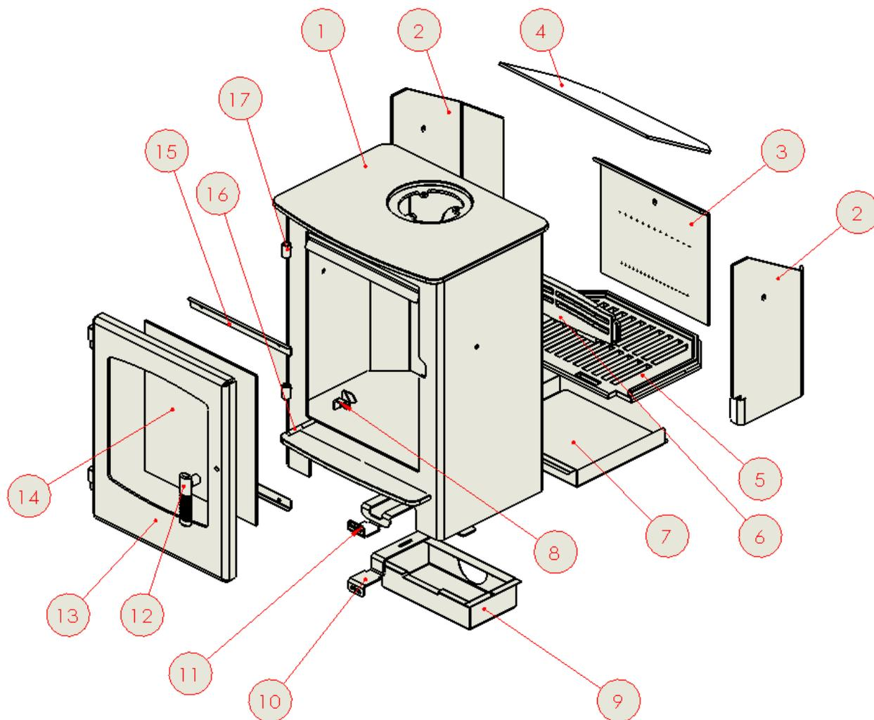
1: Stove Body. 2: LHS and RHS fire bricks, 3: Rear fire brick, 4: Baffle, 5: Grate, 6: Log retainer, 7: Ash pan, 8: Handle Latch, 9: Optional Air box, 10: Coal Slider 11: Wood Slider, 12: Door Handle, 13: Door, 14: Glass, 15: Glass Clip Top, 16: Glass Clip Bottom 17: Door Hinge
