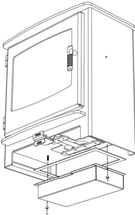
We recommend removing all loose components from inside the firebox first, the stove can then be laid on its back in order for the Air Box to be attached.
