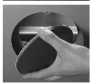
Remove any top plate, baffle plate and smoke chikane. Remove the blanking plate (3 M6 nuts) and its sealing.
