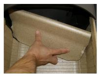
Remove the smoke chicane by lifting it up and tilting it backwards. Pull the smoke chicane out.
