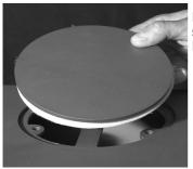
Mount the blanking plate on upper flue outlet hole - be sure to place the sealing correctly. It is all screwed together with the 3 M6 nuts.
