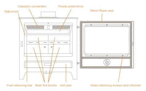
Catalytic converter cassette: This forms the "roof" of the fire box. The throat plate brick and catalytic converters are assembled in a steel "cassette". The throat plate brick can be removed without disturbing the casette.
