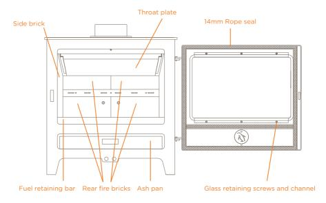
Throat plate and brick: This forms the "roof" of the fire box.
