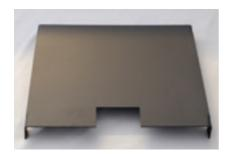
To fit: Slide in at the base of the stove prior to installation. It needs to slide in from the rear. The edge with the cut-out should slide in first, resting at the front of the stove. The folded legs of the heat shield will sit on the tabs for the leveling screws, (these are small square tabs with a hole in the centre).
