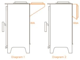
**To fit:** (if not ordered as rear flue ready) Remove both rear heat shields and blanking plate (10mm &13mm spanners required). bolt the rear adaptor to the area where the blanking plate was removed from, with the blanking plate bolts. Replace the rear heat shield, having removed the cut out with tin snips. Fit blanking disc to the underside of the stove top surface, in flue aperture.
