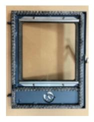
FIRE DOOR: Remove the 4 or 6 stainless steel screws retaining the double glazed glass panel. This panel is two pieces of glass with a 2mm x 10mm seal between them. Replace the 2mm x 10mm seal if necessary. Position replacement glass and fit retaining channels, tighten screws just enough to pinch the glass. Overtightening can result in the glass cracking.
