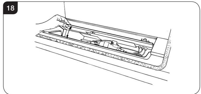
7.7 Disconnect the two cables marked 'A' in Diagram 19.
