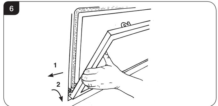
3.11 Slide the frame to the right so it comes off the right hinge pin. The window frame should now be free.
