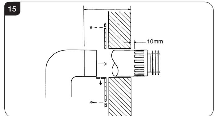
A wall plate is supplied to fix the flue to the wall:
