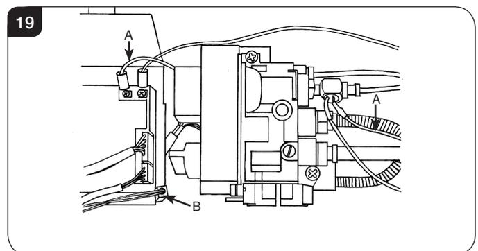
7.8 Disconnect the battery extension lead, Diagram 19, B.
