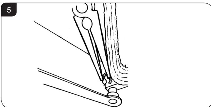
3.9 With the window frame in an upright position slide the frame to the left so that it comes off the left hinge pin, see Diagram 6 (1).
