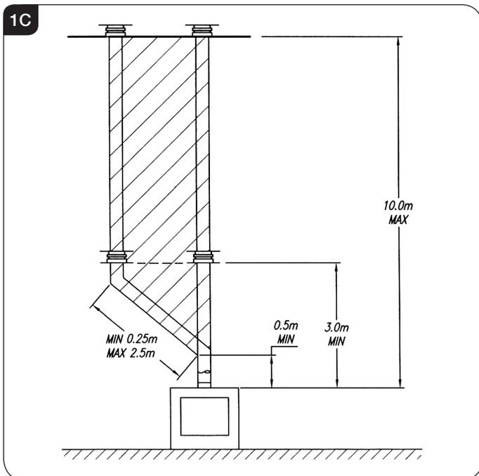
**i** This Gazco balanced flue system is designed to run internally with only the terminal projecting from the building.
