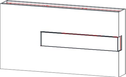
A perspective view of a fireplace unit installed in a wall. The unit is fully recessed, with its top and left side flush with the wall. The right side is open, and the front glass is exposed.                                       | <p><b>Two-Sided Installation:</b></p> <ul style="list-style-type: none"><li>• Glass exposed on the front and left or right side.</li><li>• Fireplace is fully recessed into the wall with one side open.</li></ul>        |
