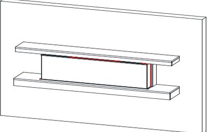
A perspective view of a fireplace unit installed in a wall. The unit is fully recessed, with its top, left, and right sides flush with the wall. The front glass is exposed. The unit is supported by a slide-in cabinet structure. | <p><b>Slide-in cabinet installation:</b></p> <ul style="list-style-type: none"><li>• Glass exposed on the left, front, and right sides</li><li>• Fireplace is fully recessed into the wall with both sides open</li></ul> |
