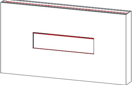
A perspective view of a fireplace unit installed in a wall. The unit is fully recessed, with its top, left, and right sides flush with the wall. Only the front glass is exposed.                                                    | <p><b>Single-Sided Installation:</b></p> <ul style="list-style-type: none"><li>• Glass exposed in the front of the fireplace.</li><li>• Fireplace is fully recessed into the wall.</li></ul>                              |
