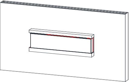
A perspective view of a fireplace unit installed in a wall. The unit is partially recessed, with its top and left side flush with the wall. The right side and front glass are exposed.                                             | <p><b>Partial Recess Installation:</b></p> <ul style="list-style-type: none"><li>• Glass exposed on the left, front, and right sides</li><li>• Fireplace is fully recessed into the wall with both sides open</li></ul>   |
