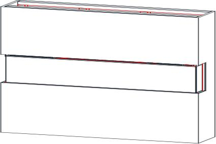
A perspective view of a fireplace unit installed in a wall. The unit is fully recessed, with its top, left, and right sides flush with the wall. The front glass is exposed.                                                          | <p><b>Three-Sided Installation:</b></p> <ul style="list-style-type: none"><li>• Glass exposed on the left, front, and right sides</li><li>• Fireplace is fully recessed into the wall with both sides open</li></ul>      |
